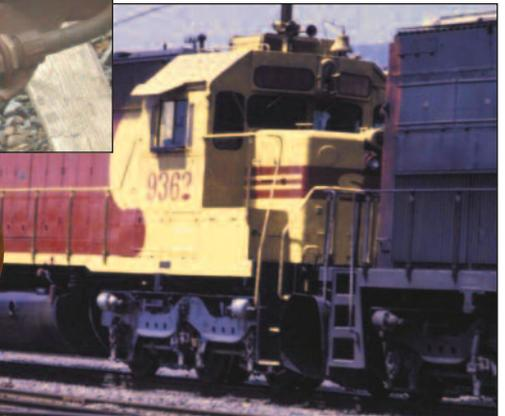
Rail cars are connected to locomotives and other rail cars by huge couplers located on each end. The couplers self-align and lock together when two cars are pushed together. A transportation company wants to measure the forces that these couplers are subjected to when the pull of the locomotive gets tons of rail cars moving from a dead stop, and while pulling the train. Additionally, the forces encountered during braking are significant as the momentum of the rail cars push against each other.
