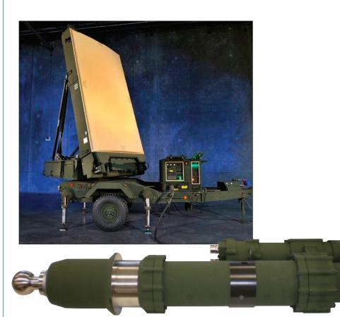
The Ground/Air Task-Oriented Radar (G/ATOR), in development by the United States Marine Corps, is a tactical radar system designed to detect, identify, and track low-level cruise missiles, manned aircraft, and unmanned aerial vehicles as well as rockets, and mortar and artillery fire. The groundbreaking G/ATOR is a highly mobile, multi-role radar system that will perform the functions of five different ground-based radars it is slated to replace.
