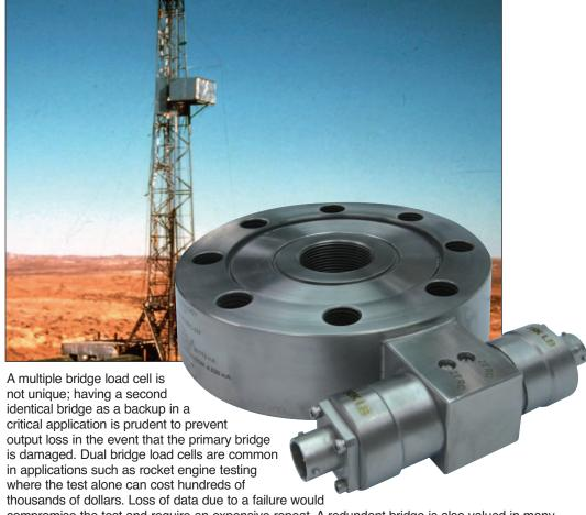
compromise the test and require an expensive repeat. A redundant bridge is also valued in many industrial and manufacturing applications where it can simultaneously provide separate outputs for both data collection and for process control.
