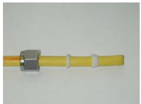
Be careful to assure proper stack up and orientation of the cable seal assembly.
