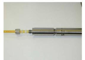
Apply thread sealant and fully tighten housing before tightening cable seal assembly.
