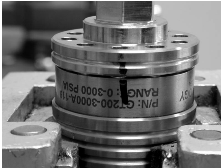
Figure 12: Re-aligning cap using marks from Step 2.
