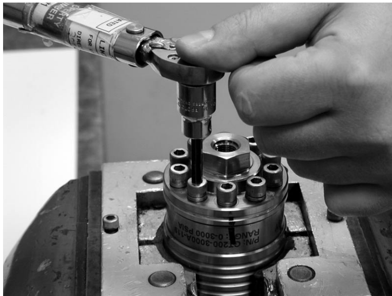
Figure 13: Setting the screw torque in proper sequence.
