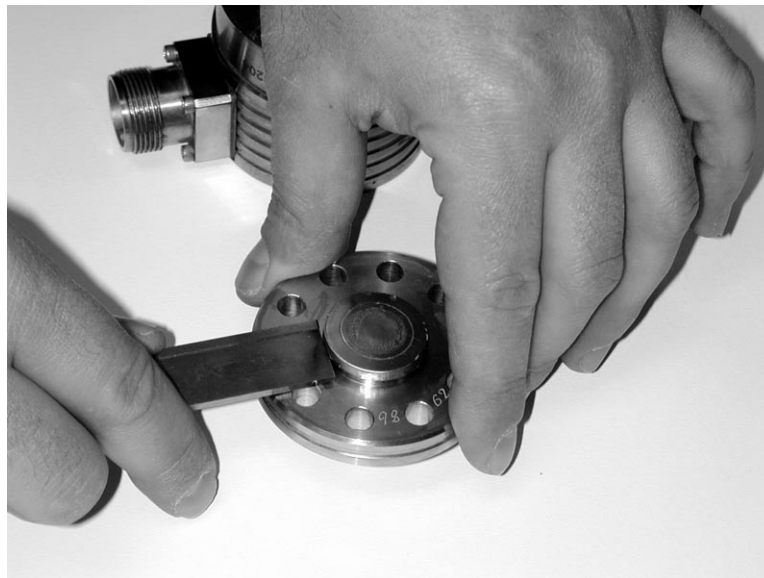
Figure 5: Removing the diaphragm.
